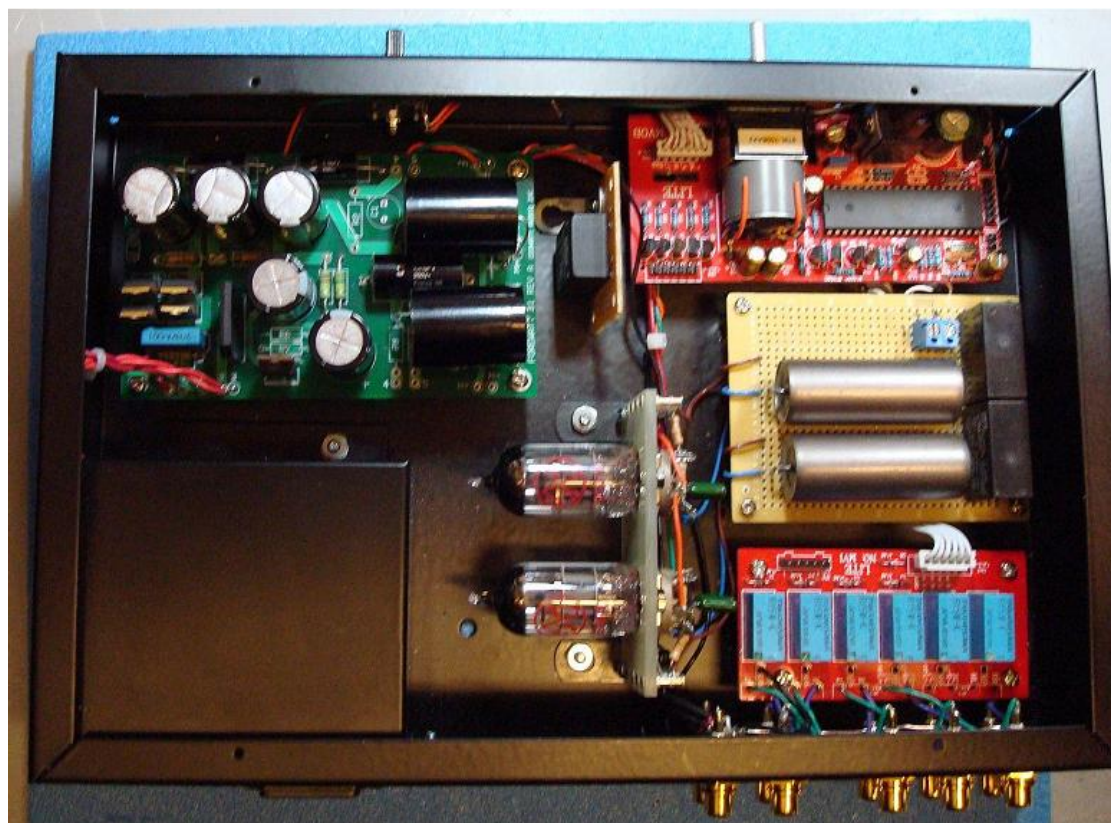
Photograph 3: ForeWatt Type II Preamp with remote control circuitry
